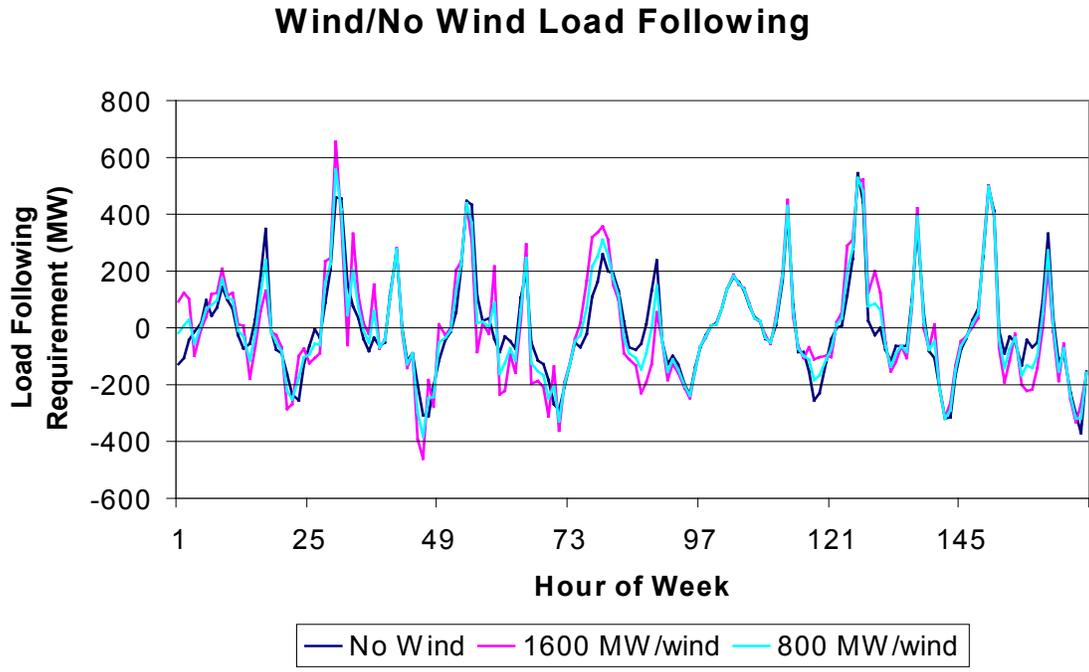
FIGURE 2. CASE 5: COMPARISON OF LOAD FOLLOWING WITH/WITHOUT WIND.
