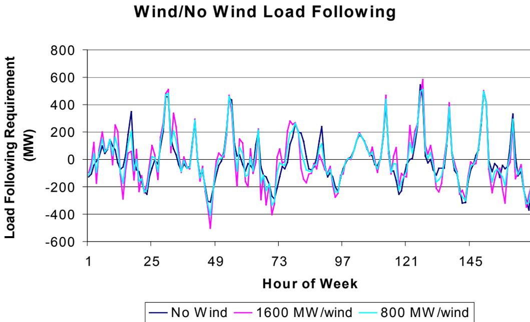
FIGURE 1. CASE 1: COMPARISON OF LOAD FOLLOWING WITH/WITHOUT WIND.
