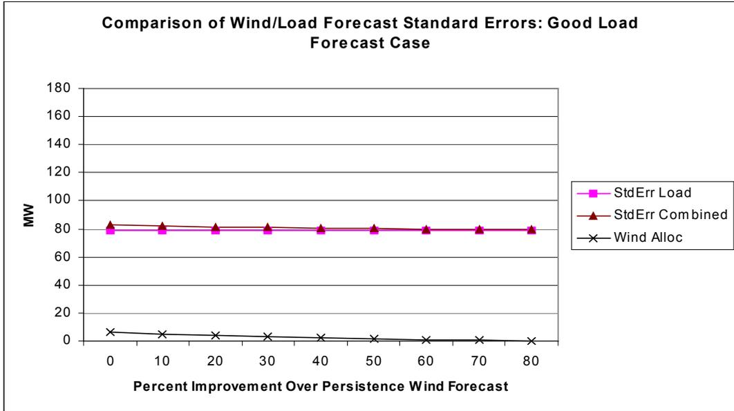
FIGURE 10. STANDARD DEVIATIONS FOR LOAD AND WIND FORECAST ERRORS COMPARED TO COMBINED FORECAST ERRORS. 400 MW WIND CAPACITY.
