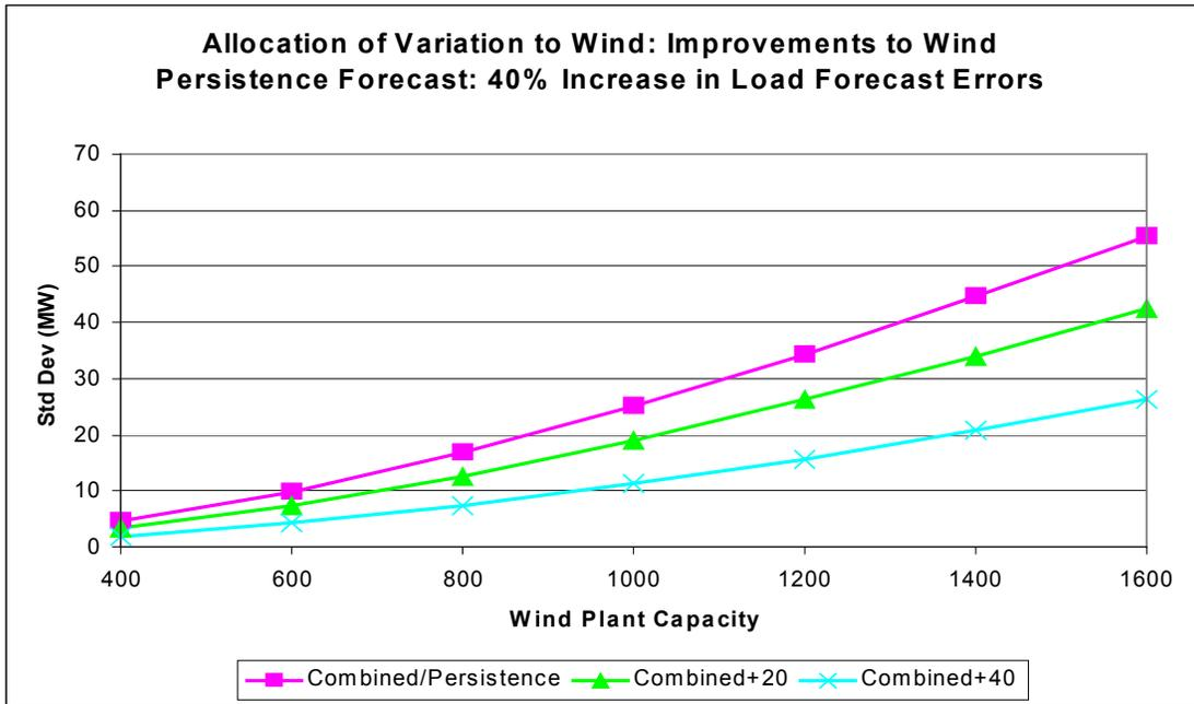
FIGURE 22. ALLOCATION OF SYSTEM IMBALANCE TO WIND FOR VARIOUS LEVELS OF WIND FORECAST ACCURACIES AND PENETRATION RATES USING ORNL VECTOR ALLOCATION METHOD. 40% DEGRADATION IN LOAD FORECAST ACCURACY.
