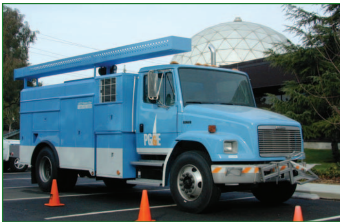
PG&E was the first company to combine a CNG engine with a heavy-duty chassis in a utility vehicle application.
