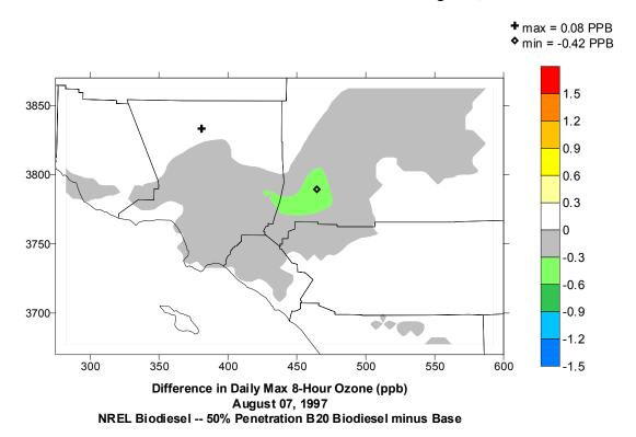
Figure D-2d. Impacts of 50% penetration of B20 biodiesel fuel on daily maximum 8-hour ozone concentrations in the South Coast Air Basin 5-km domain on August 7, 1997.
