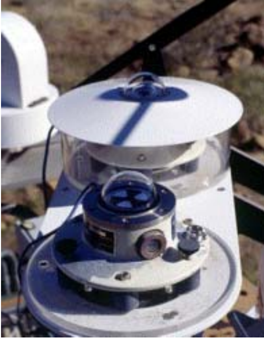
Figure 3. All-black (top unit) and black-and-white thermopile pyranometers under tracking shading disks.
