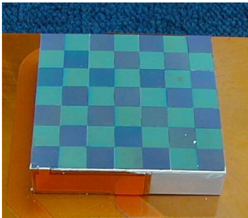
Figure 8. Amonix dense packed array.
