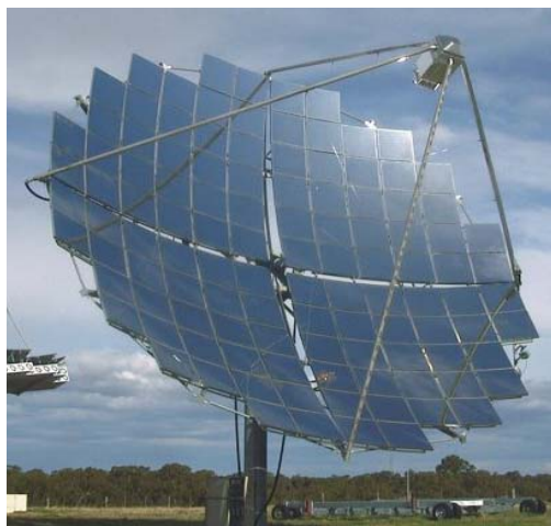
Figure 1. Solar Systems 20 kW CPV dish prototype.
