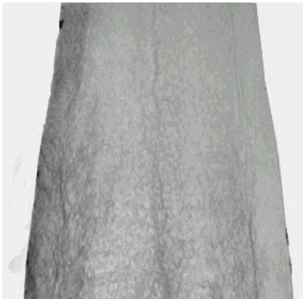
Figure 7. X-ray topograph of a dislocated Si crystal.
