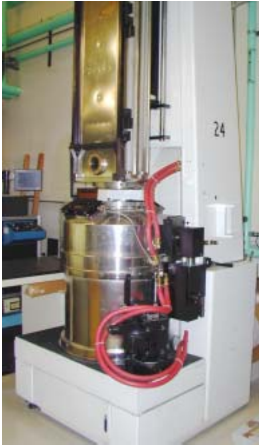
Figure 3. CZ furnace in the NREL Crystal Growth Labs.
