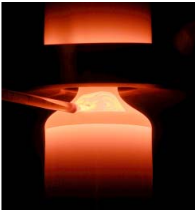
Figure 9. Solid-source oxygen doping of a 34-mm-dia., dislocation-free FZ Si crystal using a high-purity quartz rod.
