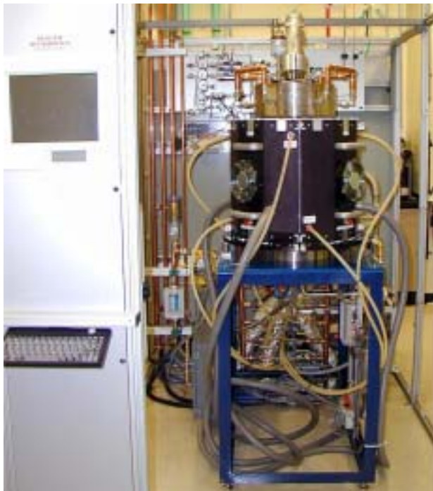
Figure 1. Silane CVD reactor for Si growth on tubes.
