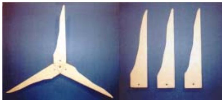
Figure 10. Blade pattern 2. Three blank blades.
