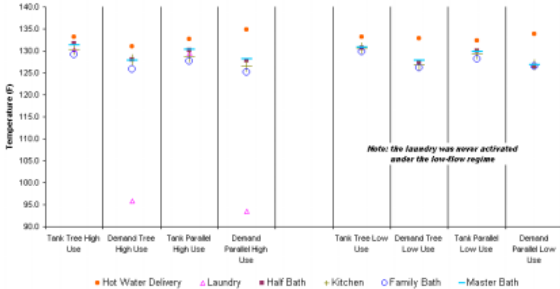
Figure 18. Experimental maximum delivery temperatures for each outlet
