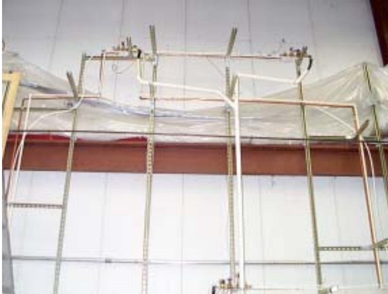
Figure 3. Partial piping system showing PEX and copper distribution systems, drains, and outlet measurement systems
