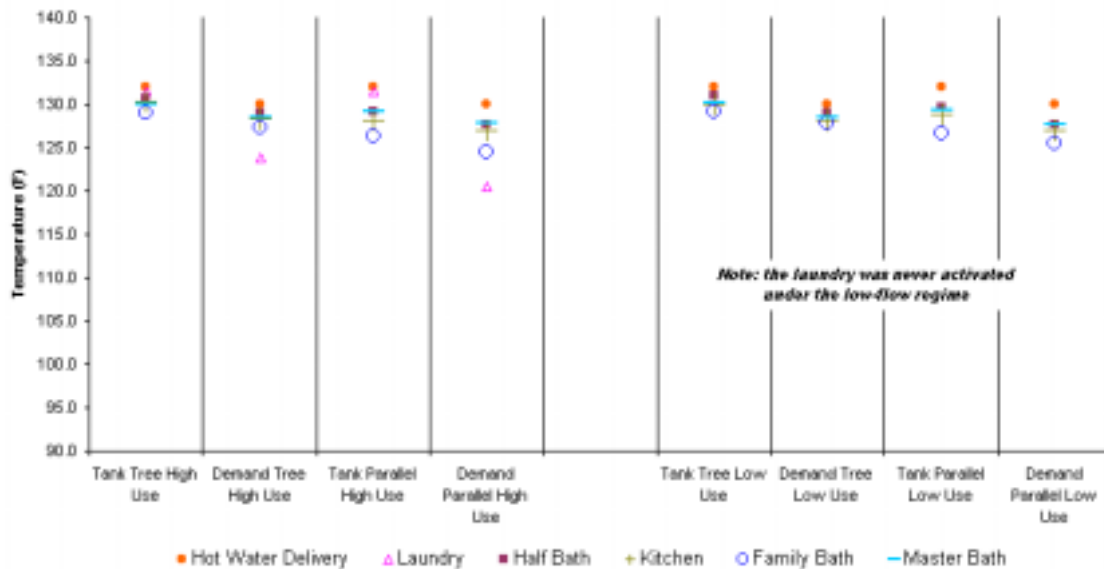
Figure 19. Simulated maximum hot water delivery temperatures
