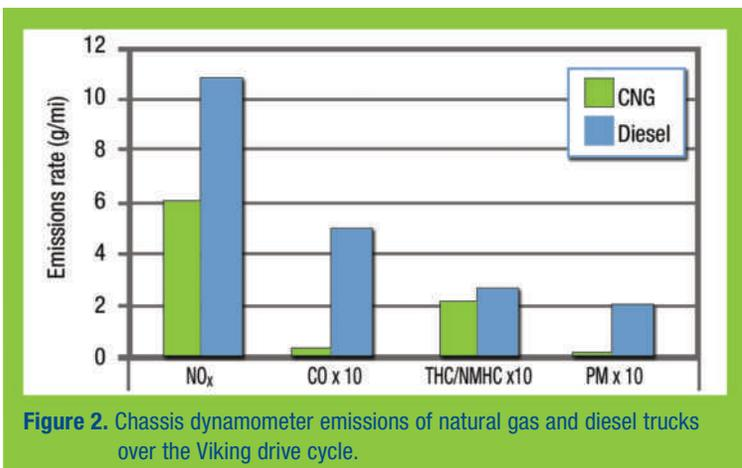
Figure 2. Chassis dynamometer emissions of natural gas and diesel trucks over the Viking drive cycle.
