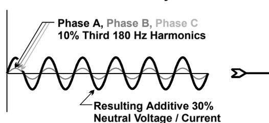
neutral due to large harmonic currents. Other symptoms may be hot and noisy transformers, short lived induction motors, and the like. In extreme cases of harmonic distortion, another symptom may be fast running electronic clocks since many of these act as a zero crossing detector of an extra harmonic voltage wave on top of the normal 60 Hertz zero crossing.
