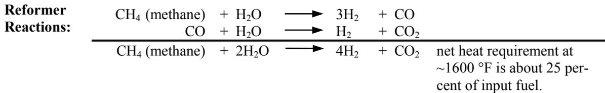
As the formula illustrates, two molecules of water (H<sub>2</sub>O) are required for each molecule of methane (CH<sub>4</sub>) in the natural gas reformer feedstock. Although this example is for natural gas, similar conversions exist for propane (C<sub>3</sub>H<sub>8</sub>) and for methanol (CH<sub>3</sub>OH) which are other common feedstocks for fuel cell power plants.
