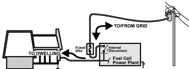
**Interconnect:** Fuel cell interconnects to the grid through a fused disconnect. An internal fuel cell disconnect is provided for certain grid parallel upsets and may be provided for certain dwelling grid independent fault clearing events.
