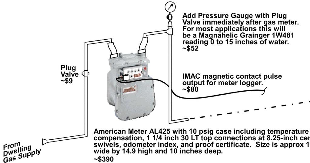
This meter may also be used for propane and can be mounted indoors or outdoors. However, preferred mounting is outdoors against dwelling wall for outdoor power plant or for propane metering. Meter can not be installed closer than three feet to any ignition source including this power plant. To preserve reasonable data collection accuracy, the meter should be installed upstream of any tubing run having material pressure losses.
