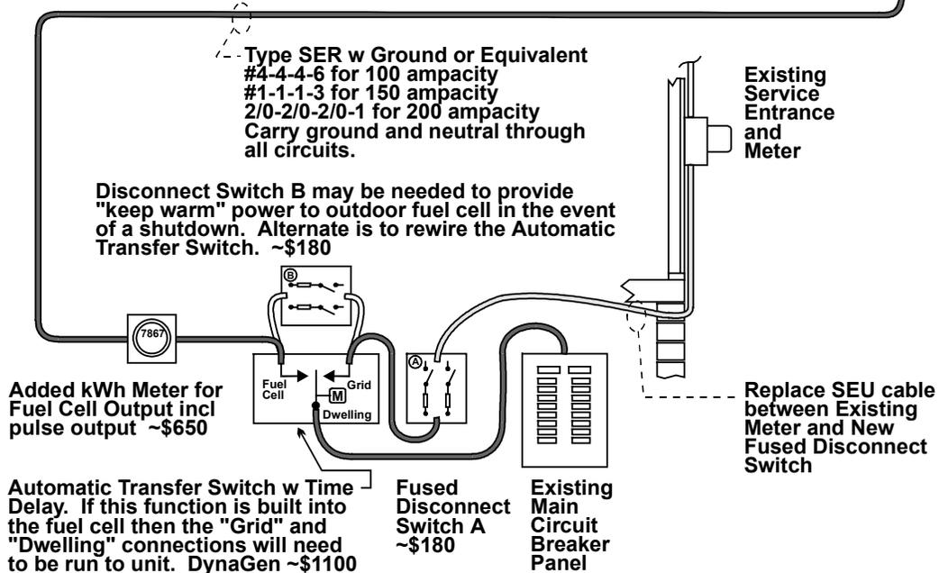
Note: Fuel cell may need separate "keep warm" circuits tied into Main Circuit Panel for outdoor freeze protection in the event of a shutdown.
