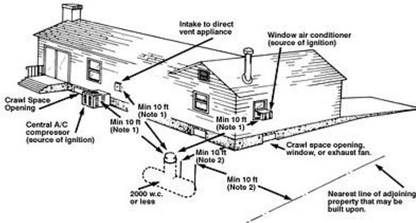
Regardless of its size, any ASME container filled on site must be located so that the filling connection and fixed maximum liquid level gauge are at least 10 ft. from any external source of ignition (e.g., open flame, window A/C, compressor), intake to direct-vented gas appliance, or intake to a mechanical ventilation system.
