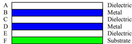
Figure 4. Schematic designs of multilayer absorber film structure.
