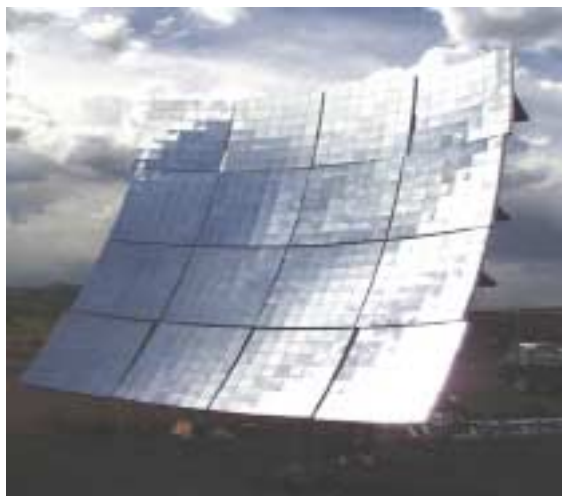
Figure 1: CTek's primary concentrator consists of more than 500 flat mirrors directed toward a secondary flux homogenizer. The system will be tested at NREL's South Table Mountain site.
