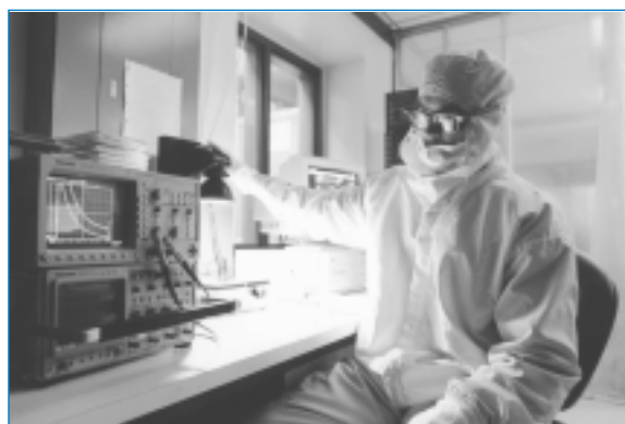
A Georgia Tech graduate student performs minority-carrier lifetime measurements by the photoconductive decay technique—important research for improving the quality of PV cells.
