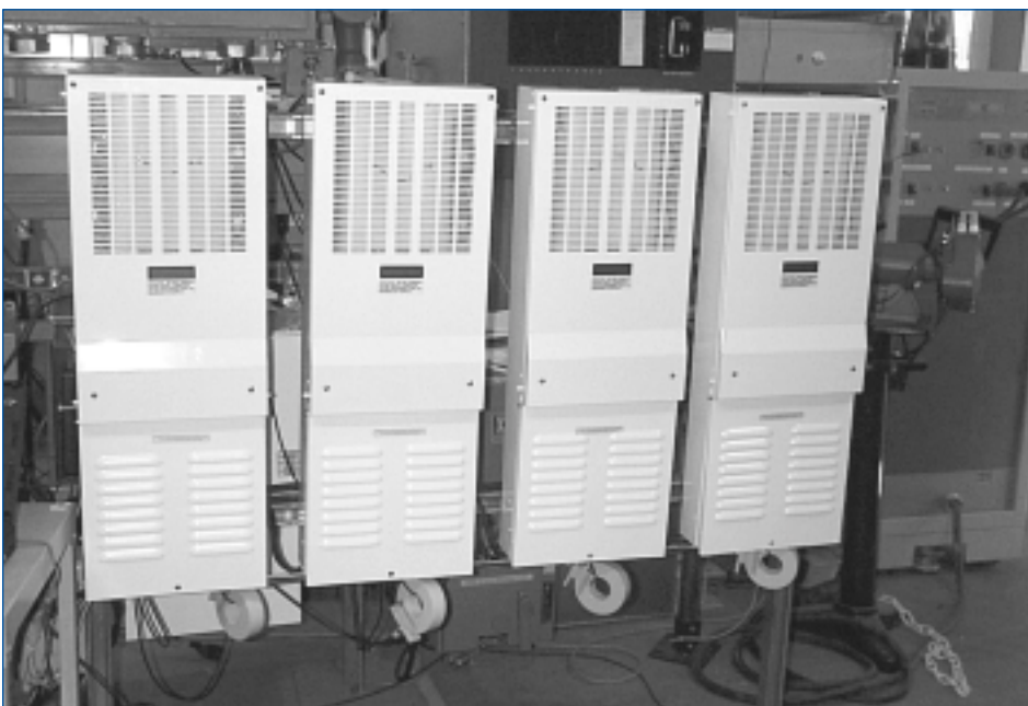
At the Sandia test bed for balance-of-systems components, four parallel Xantrex Sun Tie inverters undergo a special test for islanding requested by BP Solar.
