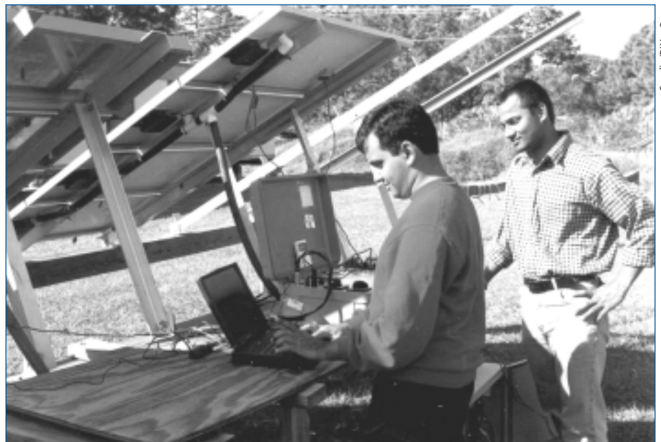
Technicians at FSEC take I-V curves of modules on the Module Long-Term Exposure Test Program. This work helps the PV industry understand performance degradation rates of modules.
