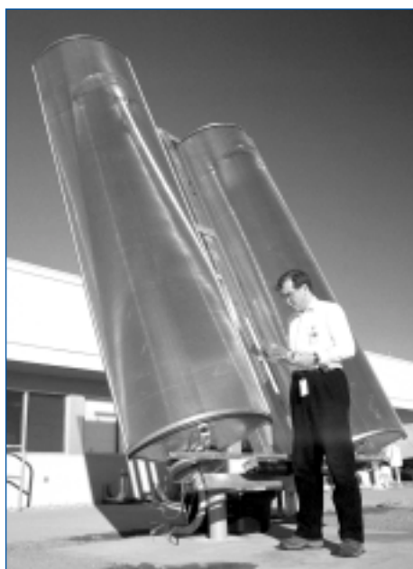
Researchers at NREL's Outdoor Test Facility in Golden, Colorado, use advanced state-of-the-art laboratories and outdoor test beds to characterize the performance and reliability of PV cells, modules, and small (1- to 5- kilowatt) systems, such as this solar concentrator system.
