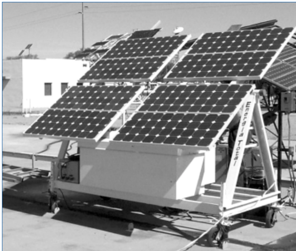
Experimental optimization of stand-alone photovoltaic systems based on ac-energy production has been made possible by integrating comprehensive module and array testing at Sandia with rapidly evolving system test procedures. Systems integrated by Energia Total, Ltd. (shown), Sacred Power Corporation, Kyocera Solar, and others are being optimized for performance and reliability.
