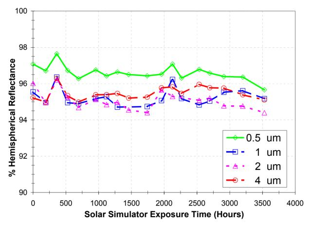
Longest durability in solar simulator of any first surface mirror
