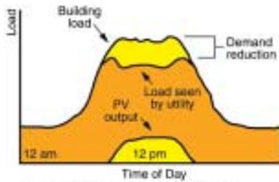
The correlation is high between commercial load (building) demand and solar availability. So PV provides power when needed, thus displacing peak energy and **reducing demand**.
