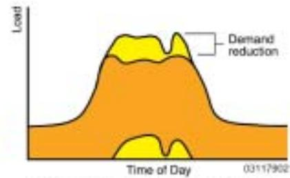
The **Solar Load Controller (SLC)** reduces the load when needed by acting on end-use settings or scheduling. Because of the naturally high correlation between PV and load, the **end-use inconvenience is minimal** compared to the demand reduction enhancement.
