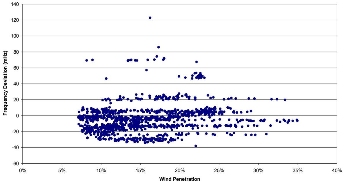
**FIGURE 8: FREQUENCY DEVIATION VS. WIND PENETRATION**
