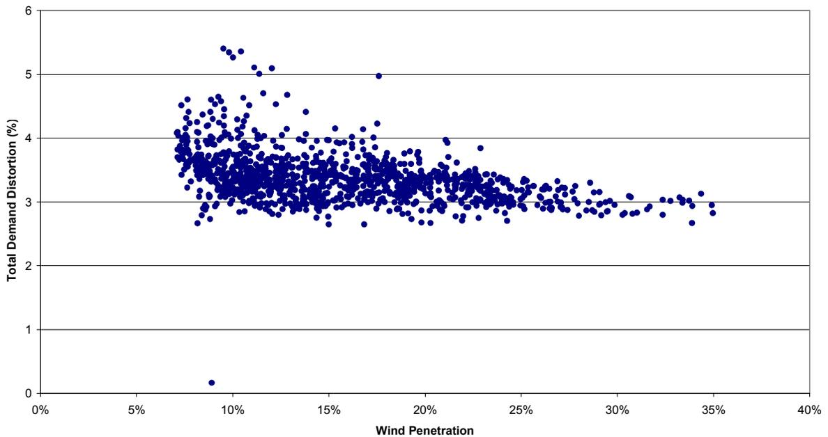
**FIGURE 7: TOTAL DEMAND DISTORTION VS. WIND PENETRATION**
