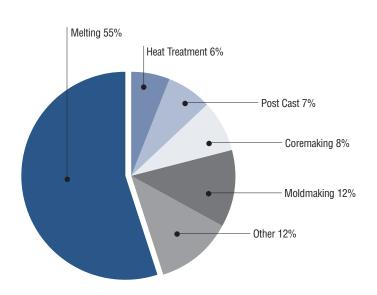
Melting is the most energy-intensive process in metal casting. Research is focusing on improving melting efficiency as well as improving yield, thereby reducing the amount of metal which must be melted.
