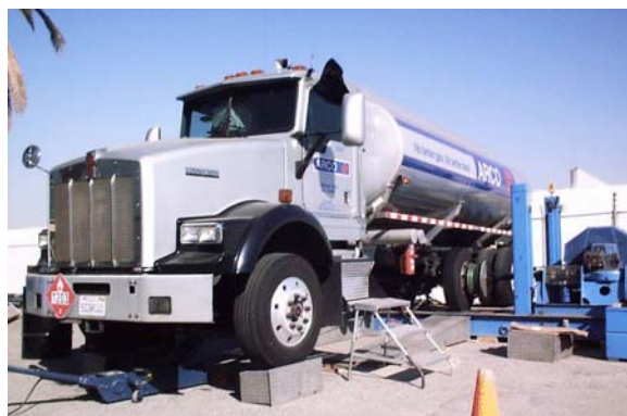
Figure 1. Tanker Truck Testing on the West Virginia University Transportable Chassis Dynamometer and Emissions Laboratory
