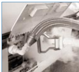
Figure 8. LNG fueling hoses connected to DART bus
