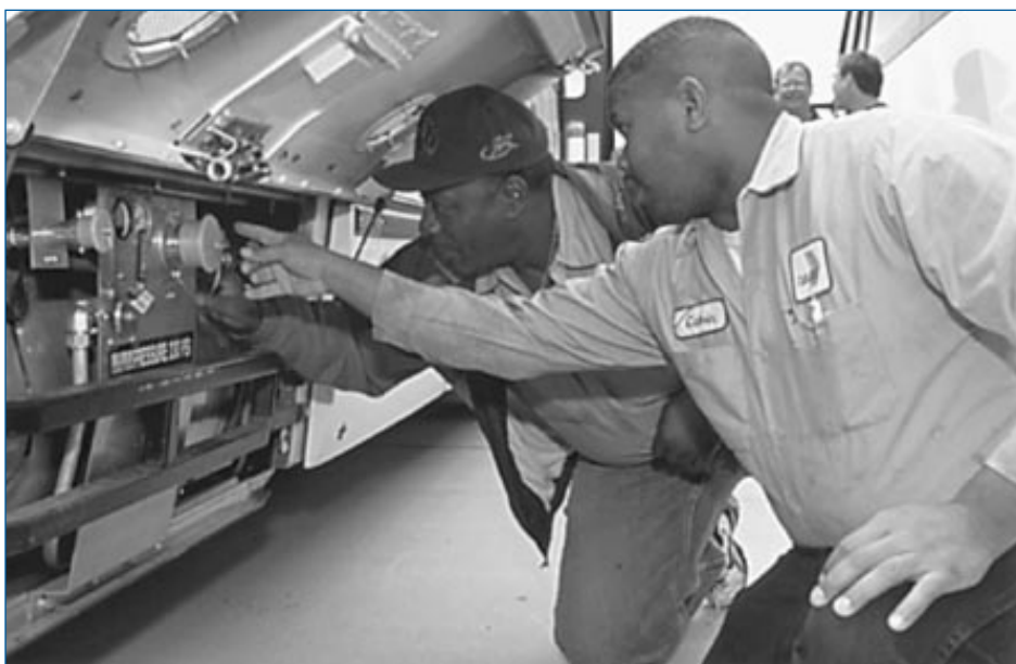
Figure 13. DART maintenance staff inspecting LNG fuel system
