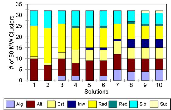
Fig. 7. Fuzzy solutions, most reliable combination of wind sites.
