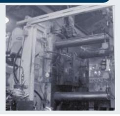
The NADCA NICE<sup>3</sup> project has developed a cleaner energy-saving method for applying lubricants during the die casting process.
