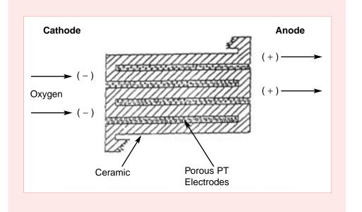
CeramPhysics' Amperometric Oxygen Sensor is a multilayer ceramic capacitor, which is ideal for inexpensive mass production and allows for miniaturization of the sensor.
