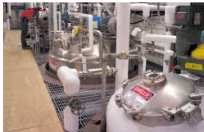
At the Bioethanol Program's one-ton-per-day Process Development Unit, bioethanol developers can test proposed processes under industrial conditions without having to build their own pilot plants.
