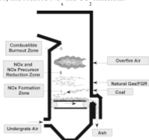
**Spreader stoker boiler retrofit with Methane de-NO<sub>x</sub> technology**
