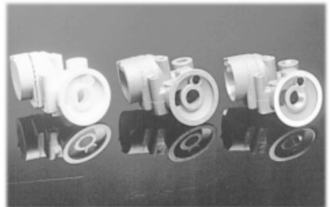
**Aluminum transmission housing produced by "lost foam process."**
