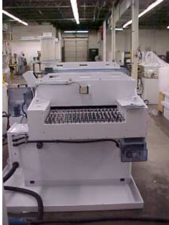
Figure 1. Continuous HF etch system – load view.
