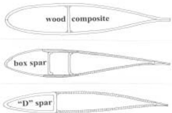
Figure 4. Large blade structural designs.
