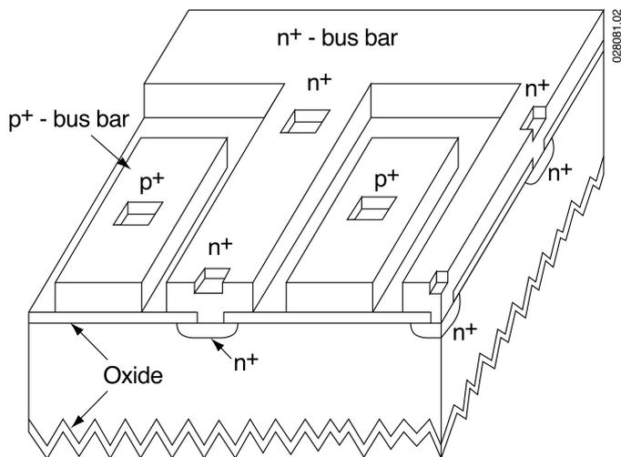
Fig. 2 Rear point contact solar cell
