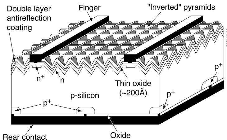
Fig. 3. Structure of the PERL cell
