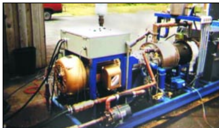
STM's gasification/Stirling engine system
