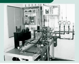
A new furnace atmosphere recovery system for steel heat treaters integrates gas membrane separation technology with a gas analysis and regeneration system that will dramatically reduce emissions, costs, and energy use.
