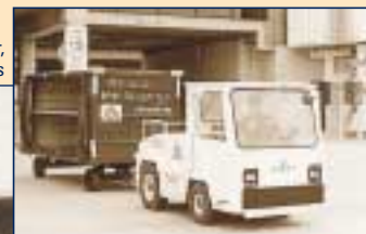
American Airlines uses electric powered baggage tractors and belt loaders at DFW
