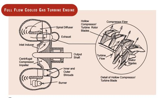
FluidTherm's innovation in turbine engines uses high-pressure air to effectively cool turbine blades, allowing the engines to reach a greater peak efficiency through increased inlet gas temperature.
