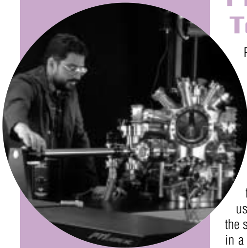
Scanning tunneling microscopy is used for imaging, three-dimensional profiling, and spectroscopic studies of material surfaces on the nanoscale and atomic levels. (Jim Yost Photography/PIX02031.)
