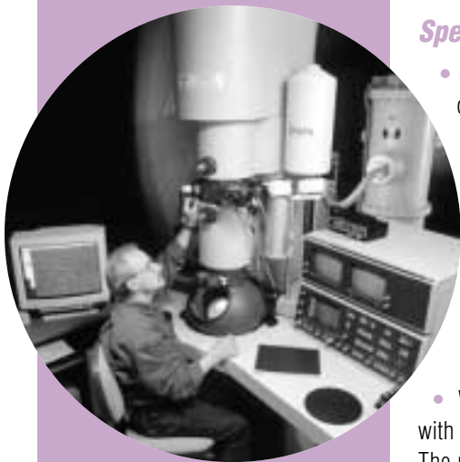
Using electron diffraction and electron imaging, the TEM/STEM analyzes the crystallographic structure, microstructure, and composition of a wide range of organic and inorganic materials. (Jim Yost Photography/PIX02016.)
