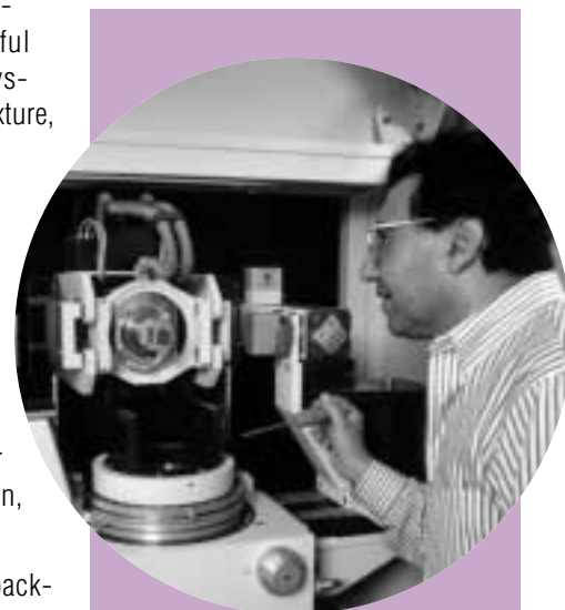
This XRD is used for identifying the crystalline phases in solid materials and powders. It also analyzes structural properties of the phases. (Jim Yost Photography/PIX04835.)
