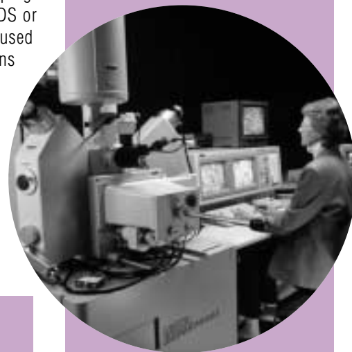
The EPMA is used to map the chemical composition of the top surface layer of solid-state materials. (Jim Yost Photography/PIX02019.)
