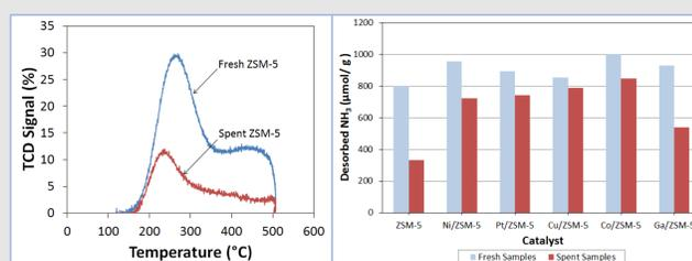
**FIG. 4.** NH<sub>3</sub>-TPD profiles of fresh and spent ZSM-5. The peaks at ~280 °C and 460 °C are due to NH<sub>3</sub> desorption from weak and strong acid sites, respectively.
