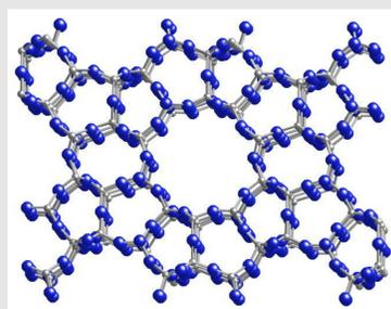
**FIG. 2.** Molecular structure of ZSM-5.
