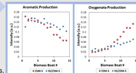
**FIG. 7.** Aromatic (benzene) vs. oxygenate (furan) production during VPU. Intensity was normalized to Ar.
