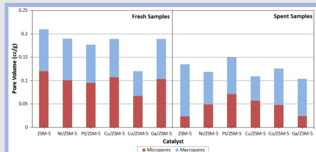
**FIG. 6.** Pore volume obtained via N<sub>2</sub>-sorption. The loss of pore volume between fresh and spent samples can be attributed to coke filling the pores.
