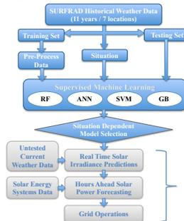
Fig 6: Big data flow from historical observations, to optimized ML models, to real time grid operations.
