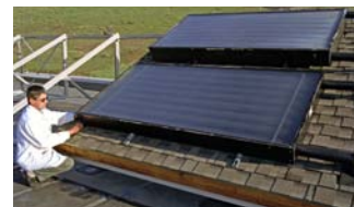
Low-cost solar collectors for cold climates are being developed and studied at the TTF's Hot Water Systems Lab. Photo by Warren Gretz, NREL/PIX 06439
