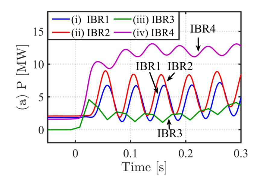
IBRs can introduce oscillatory modes into the grid.
