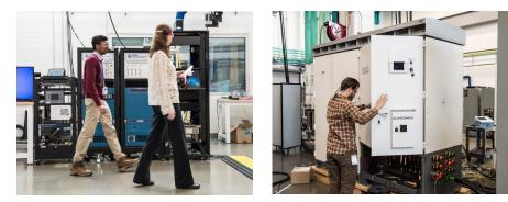
HIL test setup with real-time digital simulators, PV inverters, and advanced microgrid controllers
