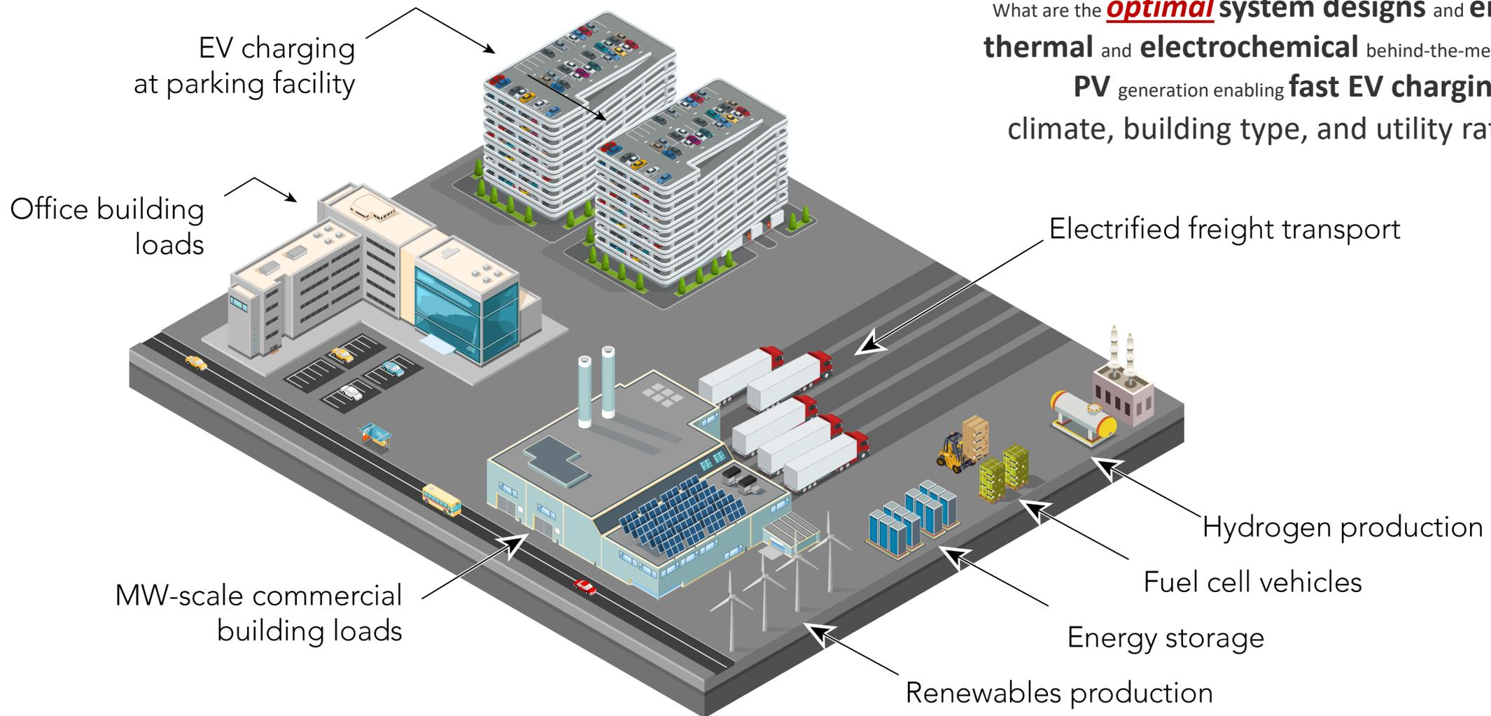
What are the ***optimal*** system designs and energy flows for thermal and electrochemical behind-the-meter-storage with on-site PV generation enabling fast EV charging if we vary climate, building type, and utility rate structure?
