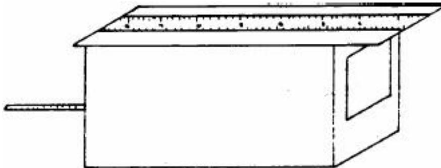
8. Place the roof so that the window is completely shaded. Wait about 5 minutes (until the temperature has stabilized) and record the temperature in the box. Also record the air temperature outside the box.
