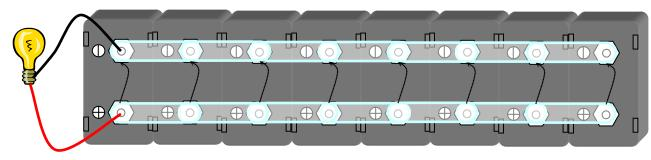
$$I_T = I_1 + I_2 + I_3 \dots \rightarrow 100 + 100 + 100 + 100 + 100 + 100 + 100 + 100 = 800 \text{ mA}$$
