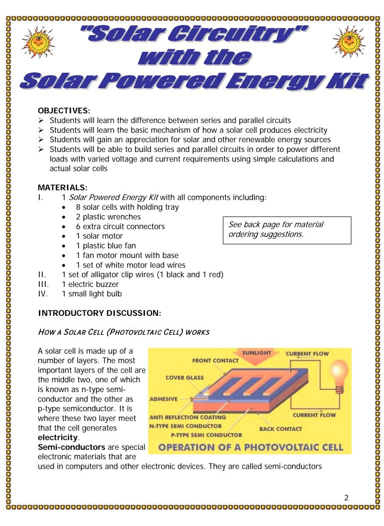
because they conduct electricity poorly when compared to metals, but they conduct very well when compared to insulators. They fall somewhere in the middle of the two. Semi-conductors have two special properties that are essential to the solar cell's ability to make electricity:
