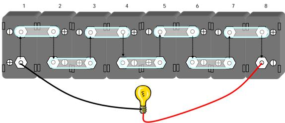
[Negative (-) and Positive (+) contacts are connected within the cell]
