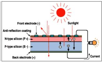
As long as light shines on the cell, we get electricity. Light comes into the cell and gets absorbed. Electrons are freed and pulled across the boundary by the electric field. They pass through an external circuit and return to their starting point.
