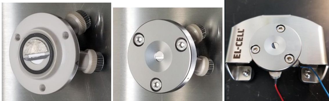
Figure 1. in-situ cell with side-by-side setup for spectroscopic analysis.
