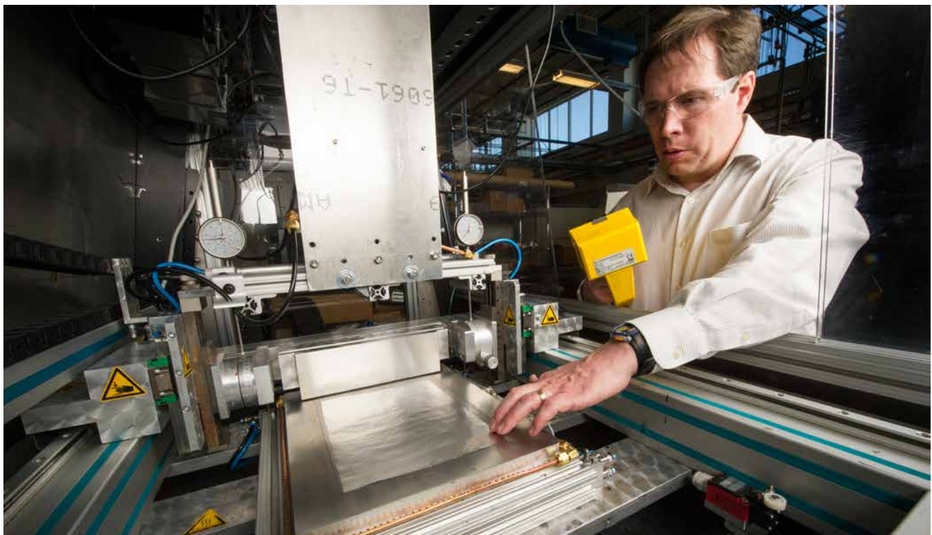
In this 2016 photo, Matt Keyser uses the slot die system in the Process Development and Integration Laboratory to coat components used in the battery internal short circuit device. Photo by Dennis Schroeder, NREL 36179
