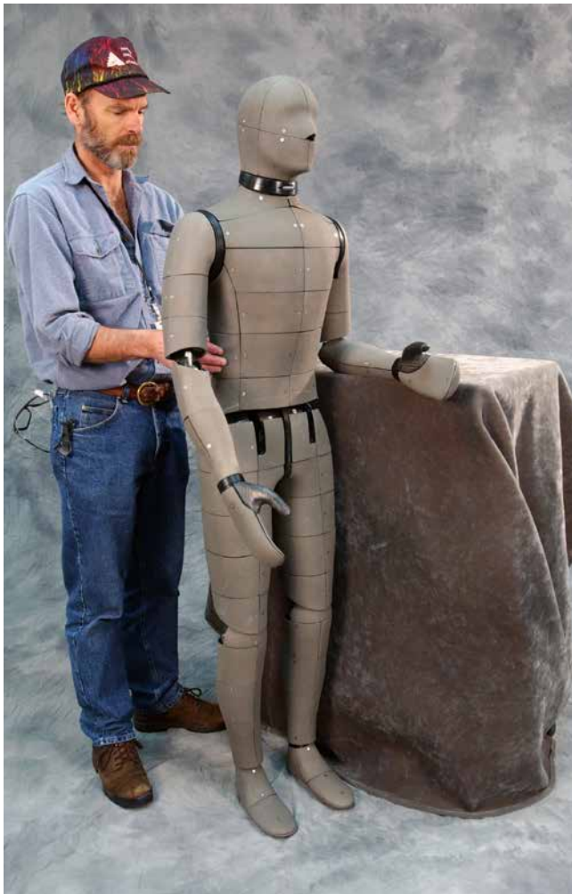
ADAM, shown in 2004, with an actual human researcher, was designed to evaluate human physiological response to thermal conditions. Sensors measure skin temperature and core temperature changes. Photo by Warren Gretz, NREL 13206
