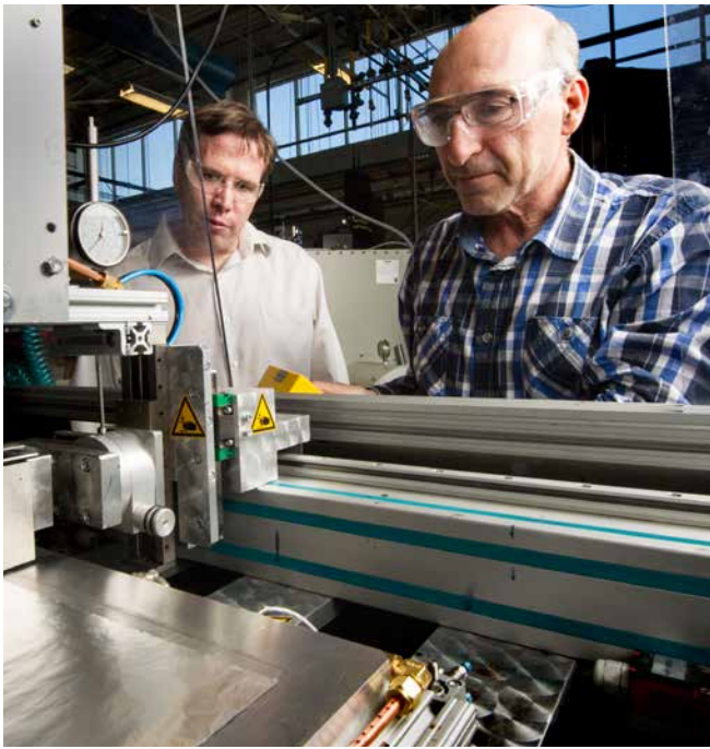
In 2016, Matt Keyser and Ahmad Pesaran worked on the battery internal short circuit device. Photo by Dennis Schroeder, NREL 36181
