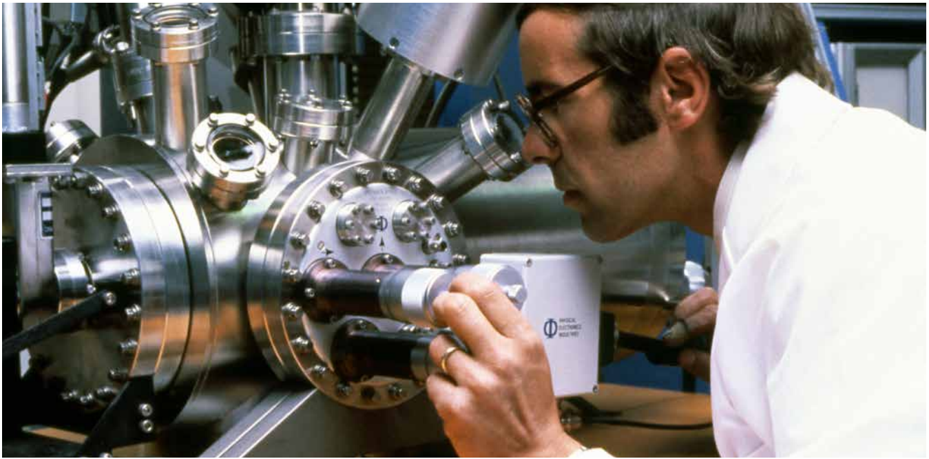
September 1996. SERI's photovoltaic research laboratories used secondary Auger and secondary ion mass spectroscopy to evaluate the compositional qualities of thin-film solar cells. Photo by Warren Gretz, NREL 00497
