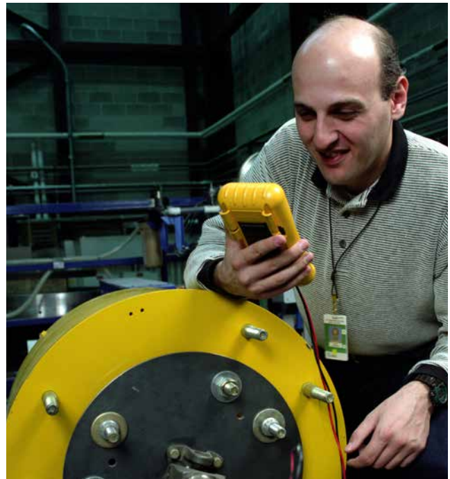
Vahan Gevorgian metering a peak power dynamometer setup with a 10-kW alternator in 1997. Photo by Warren Gretz, NREL 04759
