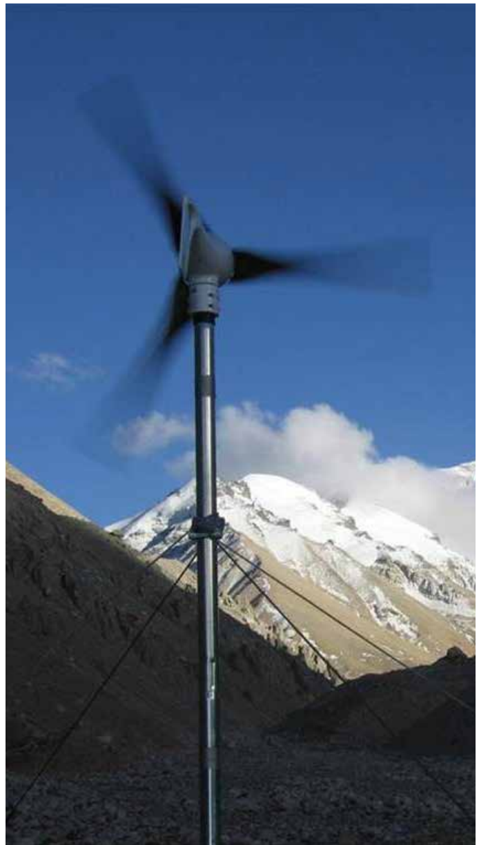
The Ryse Energy Air 30 wind turbine is one of the company's range of micro turbines. Photo from Ryse Energy LLC (formerly Primus Wind Power)
