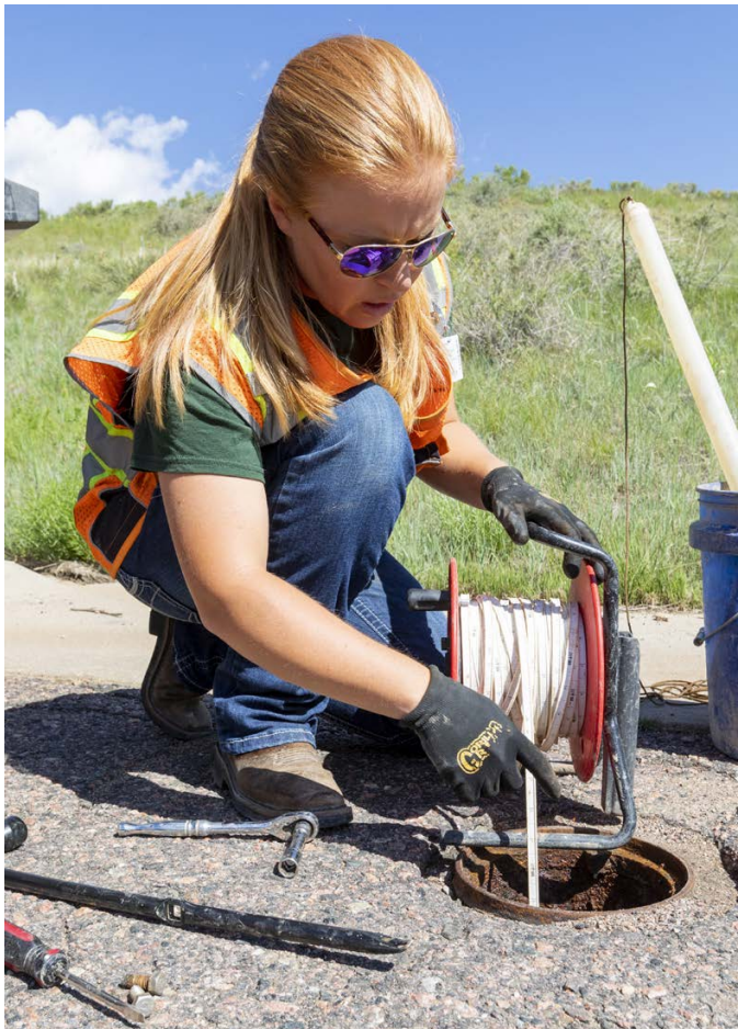
A contractor tests the water behind the Field Test Laboratory Building at the STM Campus. The wells were tested regularly to check the groundwater level, pH levels, and the total dissolved solids in the water. Photo by Werner Slocum, NREL 56795
