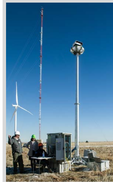
Identiflight reduces interactions between raptors and wind turbines by using cameras to curtail selective wind turbines when raptors approach. Photo by Dennis Shroeder, NREL
