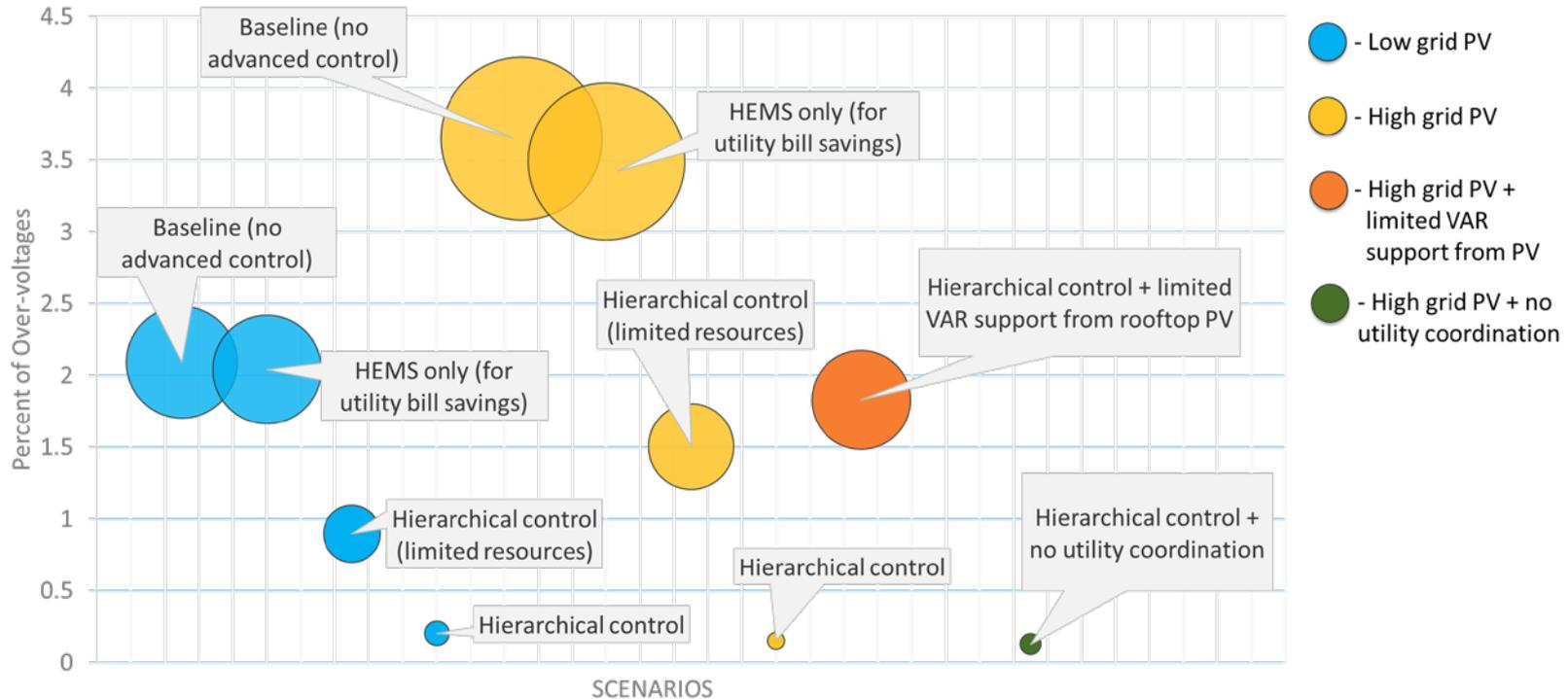
Hierarchical control algorithms successfully reduced the frequency and severity of overvoltages.
