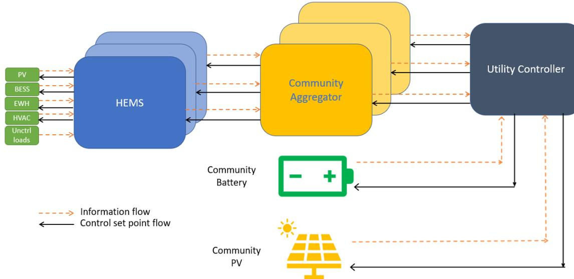
**Hierarchical control system consisting of HEMS, community aggregator, and utility controller**
