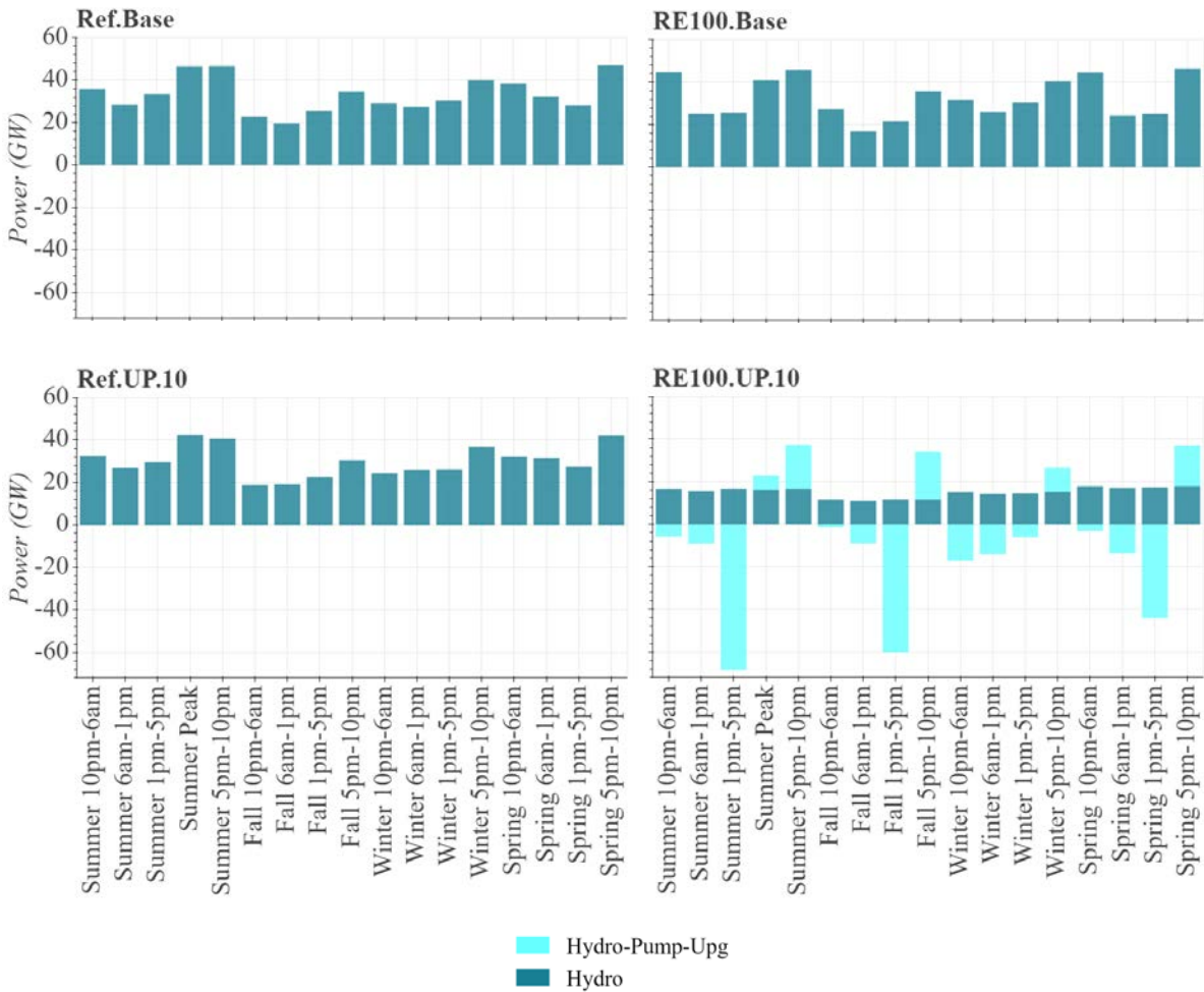
Figure 4.10. Power output from hydropower without pumping (Hydro) and hydropower with added pumps (Hydro-Pump-Upg) in each ReEDS time-slice in 2050 for Base scenarios and lowest-cost pump upgrade scenarios. Ref scenarios do not use pump upgrades for energy arbitrage, while RE100 scenarios do.
