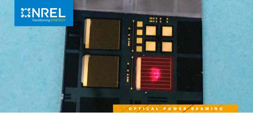
Laser beam incident on NREL-fabricated photovoltaic receiver cell. Photo by Daniel Friedman, NREL
