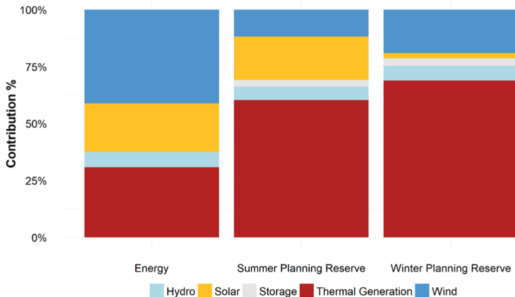
Figure 20. U.S. contribution of different technologies to energy and planning reserve in the Low Cost VG scenario
